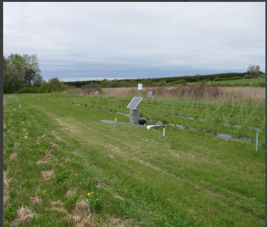
Surface Runoff Monitoring before and after plots
